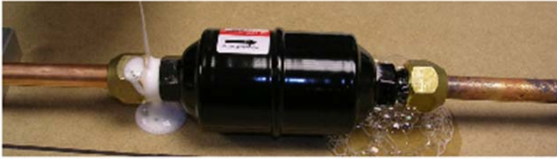
example of bubbling caused by leakage
